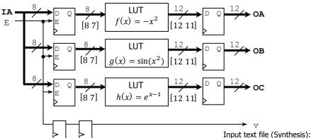
The VHDL code and testbench for this system can be found <u>here</u>.
