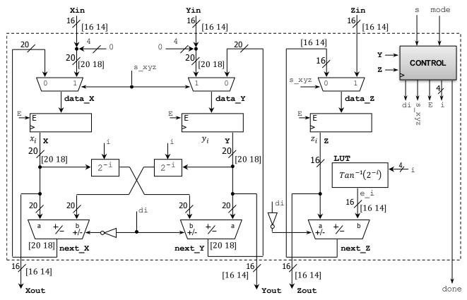
**Control**: This circuit controls the iteration index *i*, as well as the internal signals:
